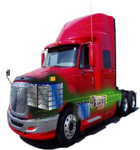
Figure 1. Conceptual layout of TransPower electric drive system in Navistar Class 8 truck.
