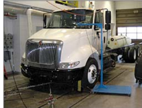
One of the trucks in NREL's B20 study is tested on the chassis dynamometer at the ReFUEL facility
