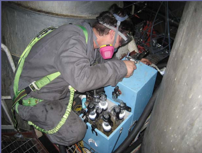
Sampling at scrubber outlet
