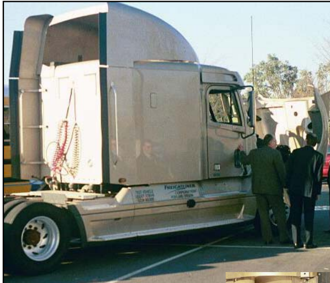
Freightliner's Century Class Tractor with DDC S60 Diesel Engine and SCR
