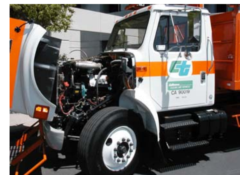
Caltrans truck retrofitted with DPF
