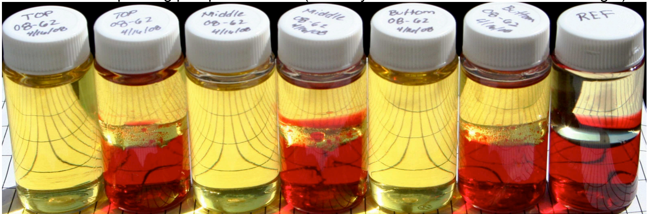
Rail Car B100 vs. corresponding pHlip Test Result (85% soy/15% FAME B100 Reference on right) at 10 min.
