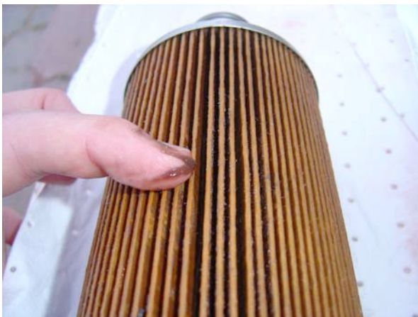
Figure 9. Bus 2210 Plugged Filter Examination
